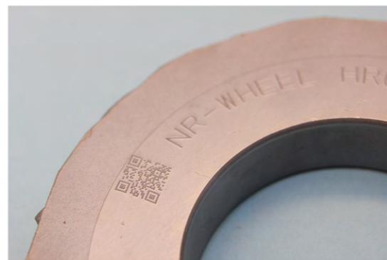
Marking on hardened parts - 62HRC.
